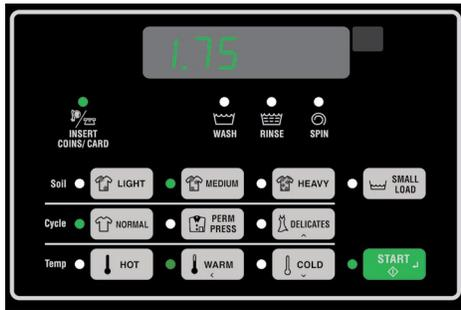
**Quantum® Control Features:** Digital display for vend price and cycle time countdown. Touch pad control with LEDs. Three temperature selections for Hot, Warm or Cold water. Three fabric selections for Normal, Permanent Press or Delicate. Extra-large capacity with small load optional. Push-to-Start activation. Infrared programming.
