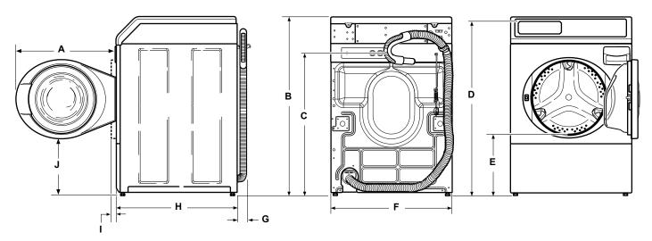
A 611 mm [24.06 in.] D 1006 mm [39.61 in.] G 52 mm [2.04 in.] J 333 mm [13.1 in.] B 1027 mm [40.42 in.] E 371 mm [14.6 in.] H 704 mm [27.73 in.] C 813 mm [32 in.] F 683 mm [26.875 in.] I (with door closed) 40 mm [1.59 in.]
